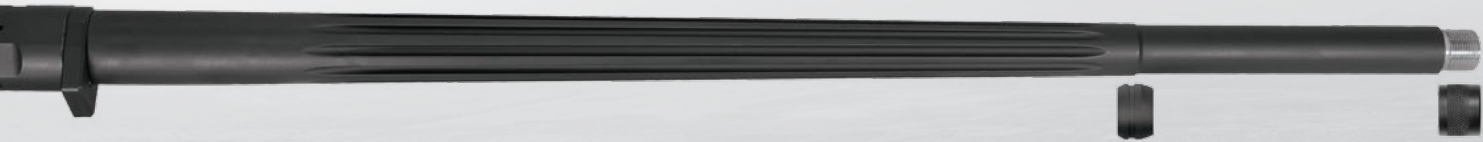
Fluted barrel - Cadex overlap suppressor ready - Optional suppressor band - Includes barrel thread protector cap - Single Point Cut rifling
