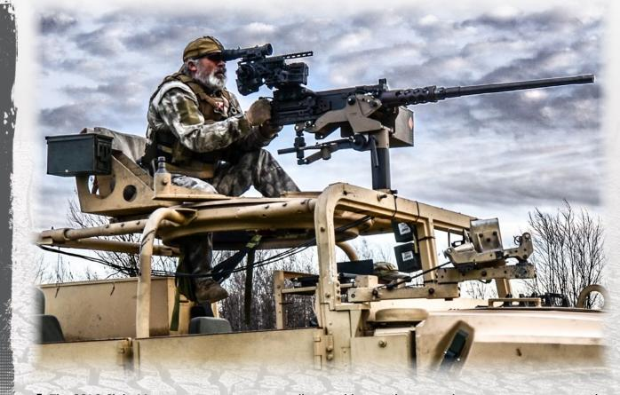
The SOLO Sight Mount converts a zone-spreading machine gun into a precise target engagement tool with one round one hit capability at extreme ranges.
